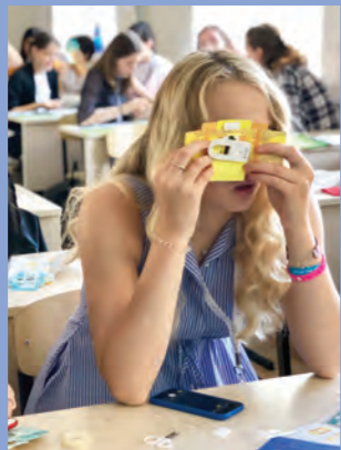
A student peers through the lens of her Foldscope, a portable paper microscope capable of 140x magnification.
