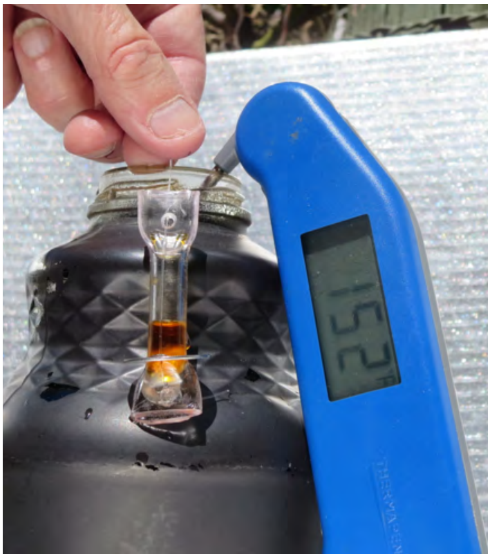
A Water Pasteurization Indicator (WAPI) indicates when the water temperature arrives at 65 degrees Celsius. Source: Robert Metcalf
