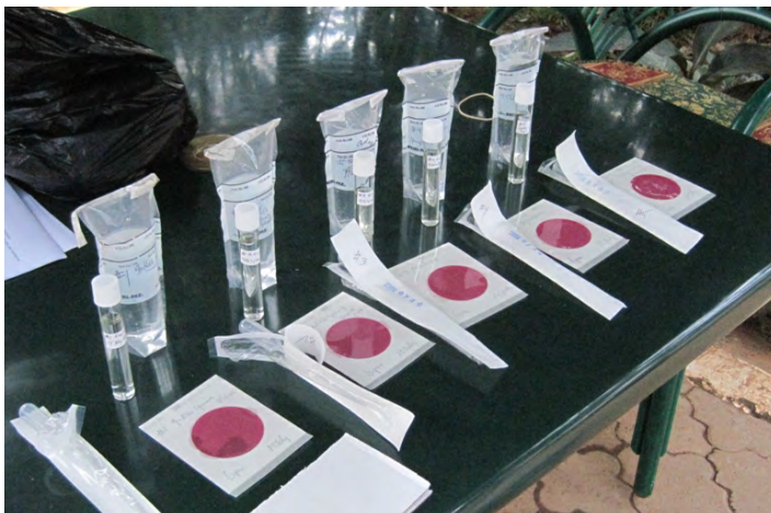
Water samples in 5 Whirl Packs are ready to be tested with Colilert 10 ml and Petrifilm tests in Kisii, Kenya. Source: Robert Metcalf
