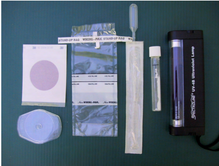
The components of a PML include a Colilert 10 milliliter presence/absence test, an E. coli count Petrifilm, a plastic spreader, a sterile collecting bag, a sterile plastic pipette and a long-wavelength UV light. Source: Robert Metcalf
