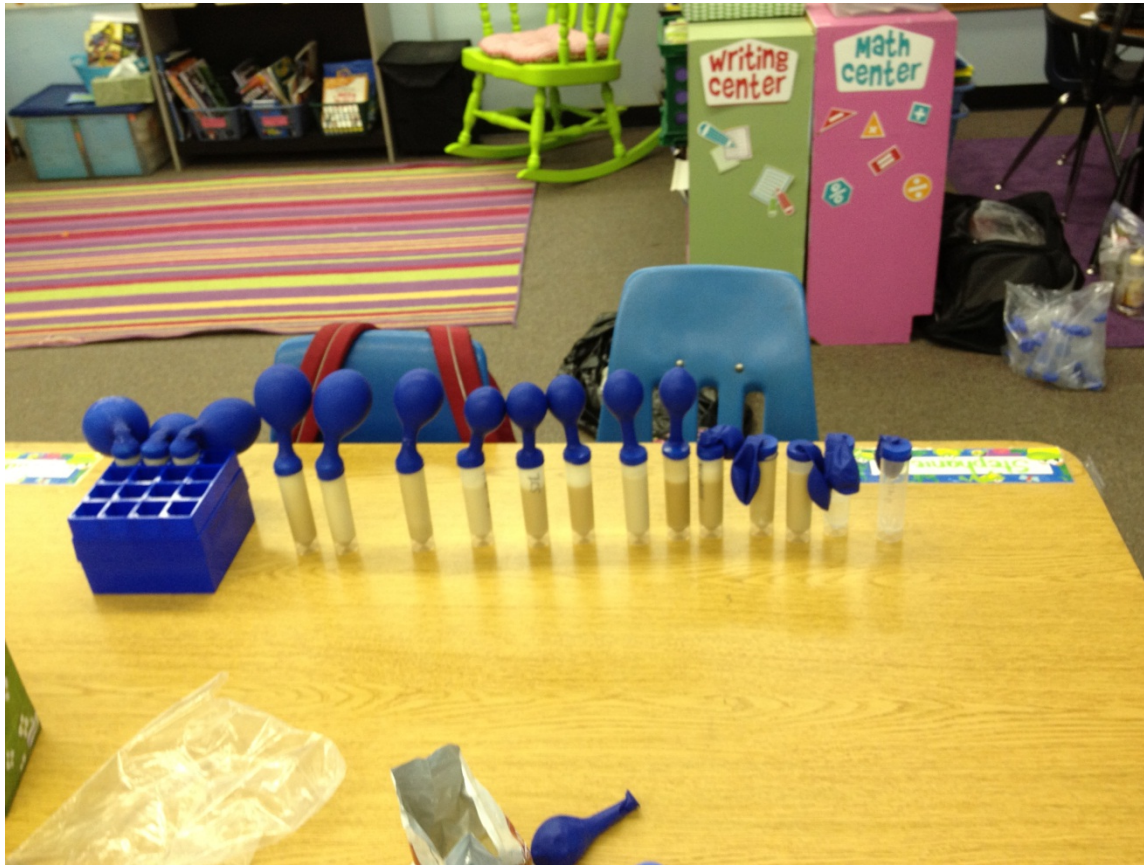
Figure 1: Students Analyzed Balloon Size as a Measure of Yeast Growth. Balloons were organized into four categories, with “3” demonstrating the most growth and “0” no growth, as measured by balloon size. Students grouped the tube/balloons from “3” (left most in test tube rack) to “0” (on right side).
